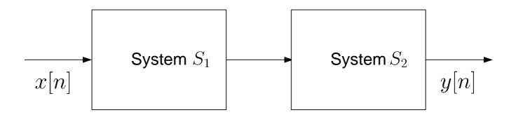
3. Determine whether the following discrete-time system, with input signal x[n] and output signal y[n] is memoryless, invertible, stable, causal, linear, and/or time-invariant:
