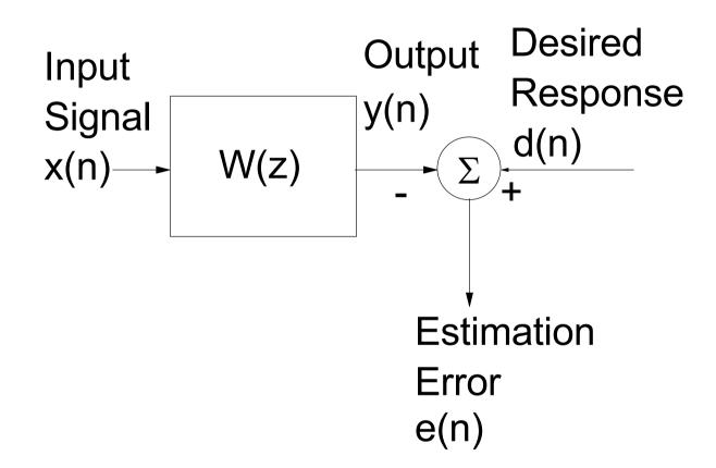
Given the input x(n) and the desired response d(n), we want to find the transfer function W(z) or its impulse response such that a statistical criterion or a cost function is optimized.
