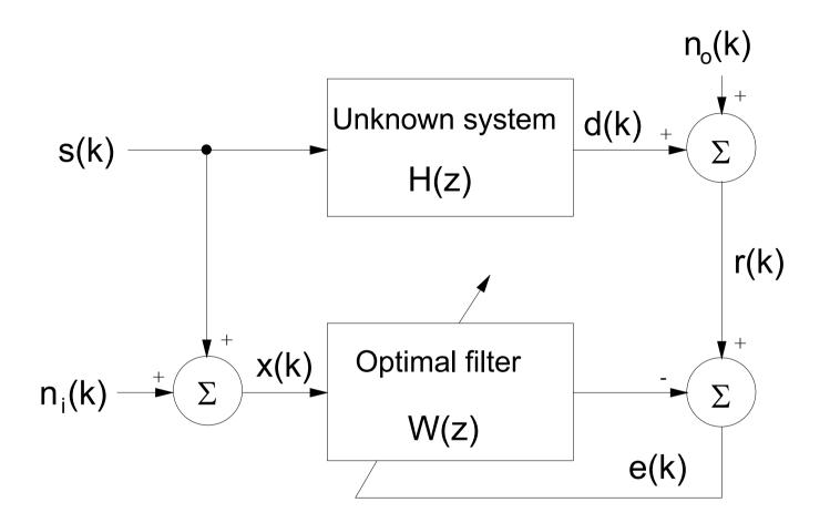
Given noisy input x(k) and/or noisy output r(k), our aim is to determine the impulse response of the unknown system H(z) using W(z)
