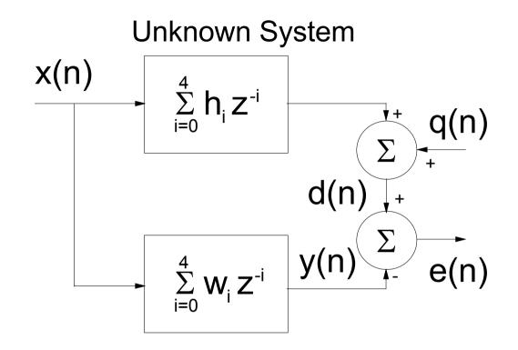
In this example least squares filtering is applied in determining the impulse response of an unknown system. Assume that the unknown impulse response is causal and  $\{h_i\}=\{1,2,3,2,1\}$ . Given *N* samples of x(n) and d(n) where q(n) is a measurement noise.
