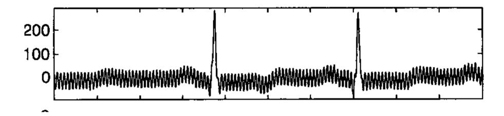
Suggest methods to eliminate/reduce the 50Hz interference.
