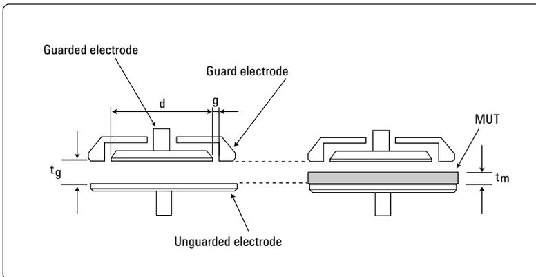
Figure 6. Non-contacting electrode method
