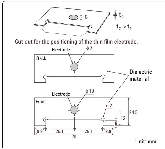
Figure 23. Fabricated thin film electrode's size
