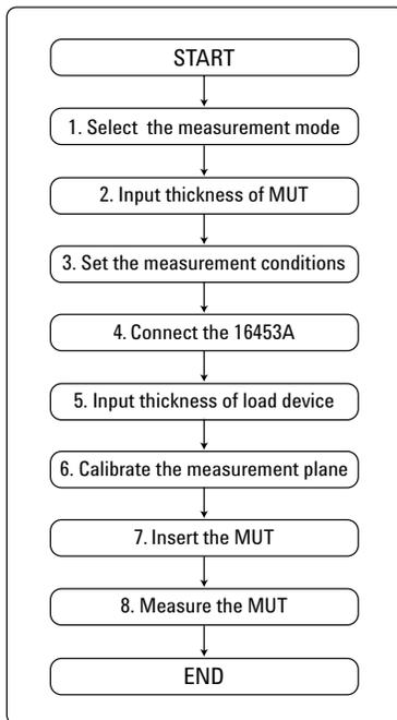
Figure 21. Measurement procedure flowchart for the 16453A
