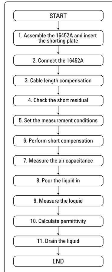
Figure 42. Measurement procedure flowchart for the 16452A
