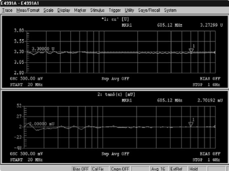
Figure 25. Frequency response of BT resin
