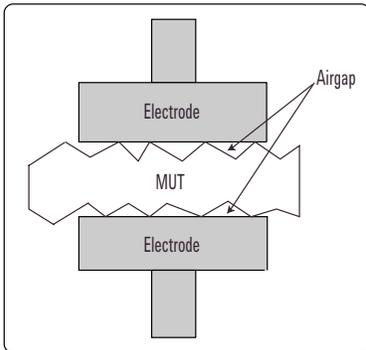
Figure 22. Rough-surfaced dielectric material
