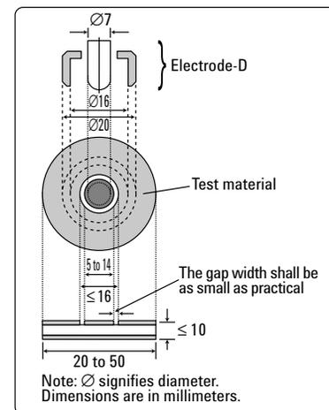
Figure 10. Electrode D dimensions
