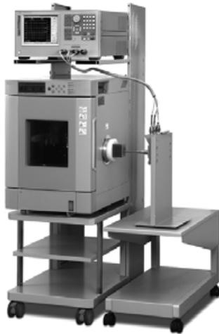
\* For temperature-response evaluations, Option E4991A-007 is required. A heat-resistant cable, that maintains high accuracy and a program for chamber control and data analysis, are included with Option E4991A-007. The 4294A does not have a high temperature test head.
