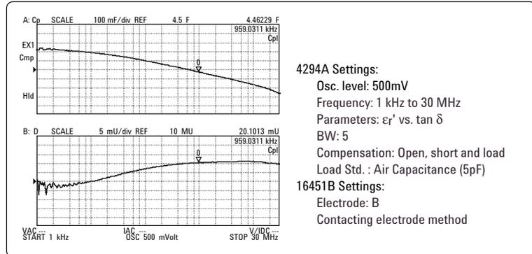
Figure 15. Frequency response of printed circuit board
