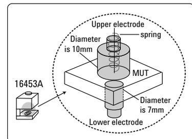
Figure 18. Structure of 16453A
