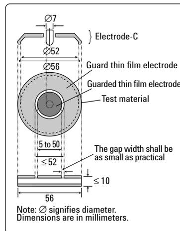
Figure 9. Electrode C dimensions
