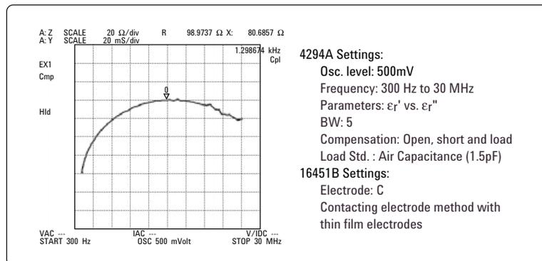
Figure 16. Cole-Cole plot of a ceramic material
