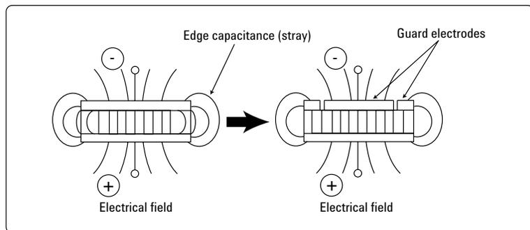
Figure 3. Effect of guard electrode
