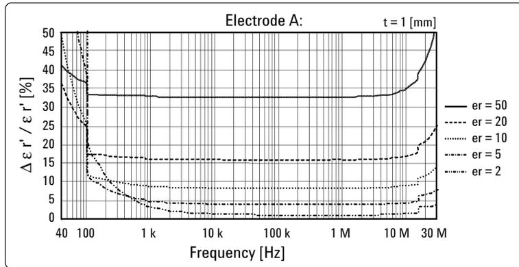
Figure 12. Permittivity measurement accuracy (supplemental data)
