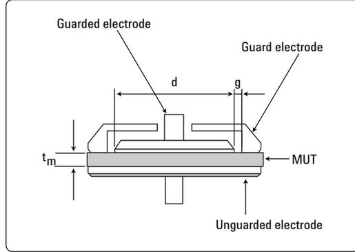
Figure 4. Contacting electrode method
