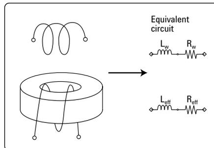
Figure 27. Method of measuring effective permeability
