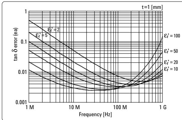
Figure 20. Loss tangent measurement accuracy (supplemental data)
