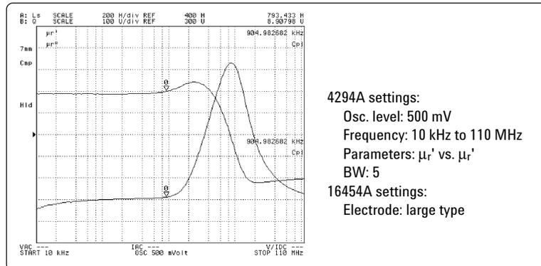
Figure 34. Low frequency response of MnZn ferrite core
