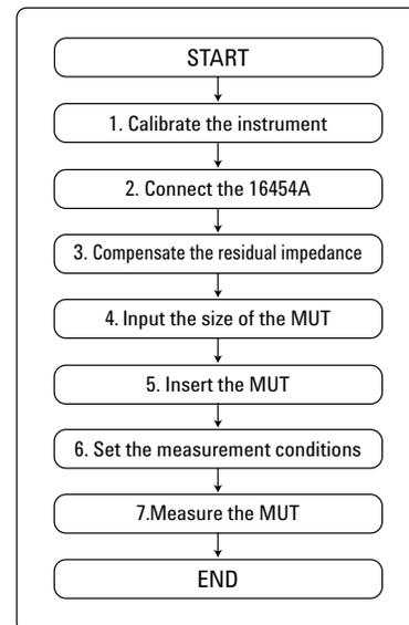
Figure 32. Measurement procedure flowchart for the 16454A
