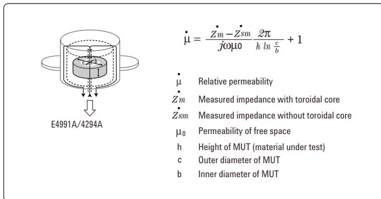
Figure 29. Structure of 16454A and measurement concept
