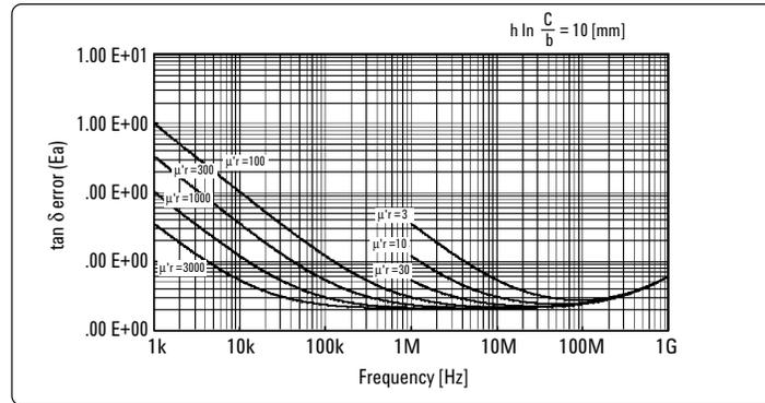
Figure 31. Loss tangent measurement accuracy (supplemental data)
