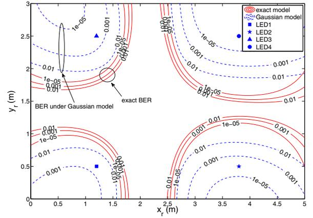
Fig. 2: The contour plot of BER for levels of  $10^{-5}$ ,  $10^{-3}$ ,  $10^{-2}$  over the  $(x_r, y_r)$  plane under the exact analysis and the Gaussian interference model.
