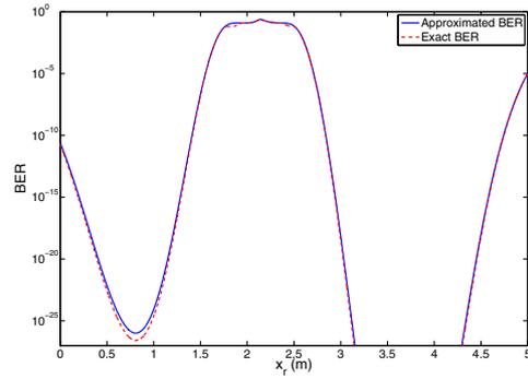
Fig. 4: The exact BER and the approximate BER. The receiver's location is  $(x_r, 0.5, 0.83)$ , i.e., on the straight line from  $LED_1$  to  $LED_2$ .
