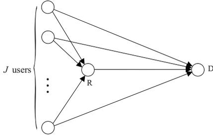
Fig. 1. The multiple access relay channel model.
