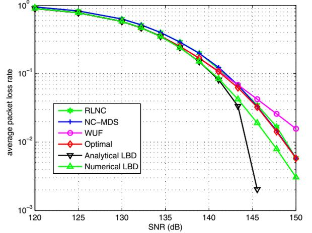
Fig. 3. Average packet loss rate comparison among WUF, NC-MDS, Optimal, two lower bounds, and RLNC,  $J = 20$ ,  $S = 1$ .
