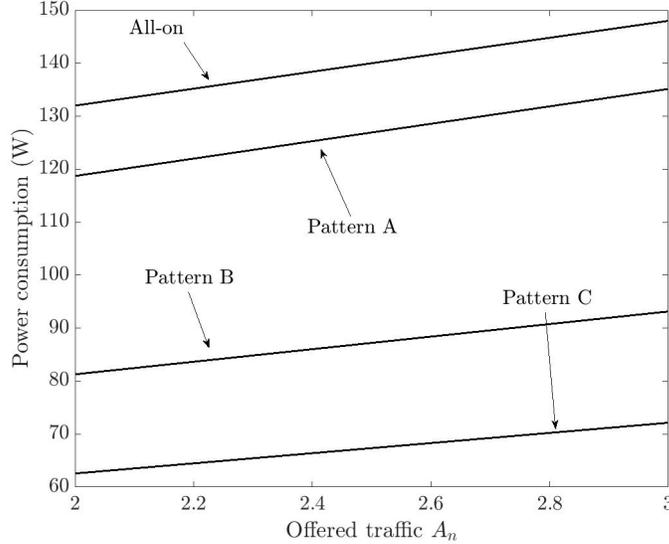
Figure 4: Average power consumptions achievable for different switching patterns.
