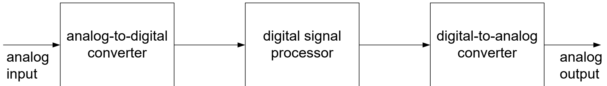
Fig.1.12: Digital processing of analog signal
