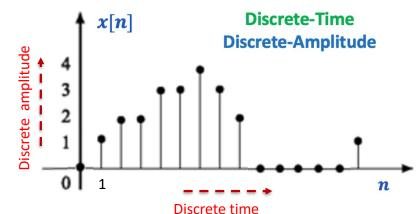
• The digital signal is the sampled and quantized (rounded) representation of the analog signal. A digital signal consists of a sequence of samples, which in this case are integers: 0, 1, 2, 2, 3, 3, 4, 3, ...
