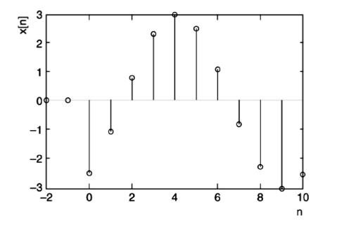
Right-Sized Periodic Sinusoidal Sequence with right shifted by one sample
