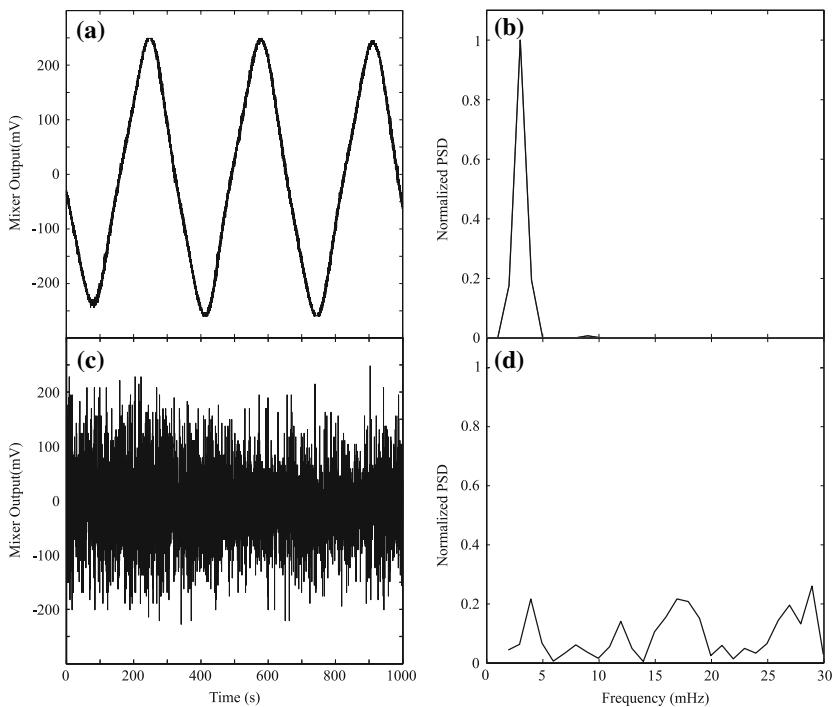
**Fig. 5** Mixer output for  $f_{\text{RF}} = 17 \text{ GHz}$ . The target moves away from the detector at  $26 \mu\text{m/s}$ . The Doppler shift frequency is  $3 \text{ mHz}$ : (a) Doppler measurement with locked period-one state, (b) the corresponding normalized power spectrum (PSD), (c) Doppler measurement with unlocked period-one state, and (d) the corresponding normalized PSD
