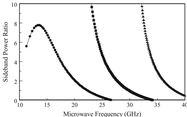
**Fig. 3** Optical power ratio of the generated sideband to the carrier. The injection strength is varied to tune the microwave frequency while the injection detuning is kept at 10 GHz (●), 20 GHz (▀), and 30 GHz (▲), respectively
