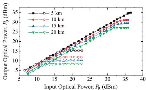
Fig. 3. (Color online) Output optical power versus input optical power for transmission over fibers. The fiber lengths are indicated by the legends. The open and closed symbols are obtained when the slave laser is in the free-running state and the chaotic state, respectively. For each curve, the output power saturates because of SBS reflection.
