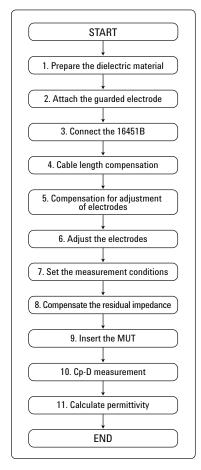
Figure 14. Measurement procedure flowchart for the 16451B
