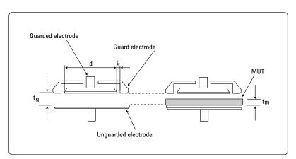
Figure 6. Non-contacting electrode method
