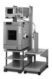
\* For temperature-response evaluation, Option E4991A-007 temperature characteristic test kit is required. A heat-resistant cable, that maintains high accuracy, and a program for chamber control and data analysis are included with Option E4991A-007.
