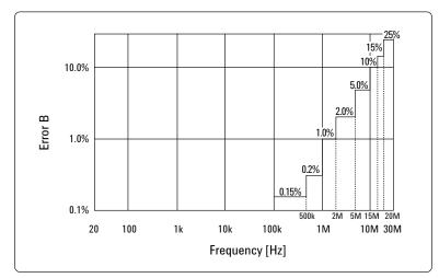
Figure 41. Relative measurement accuracy (supplemental data)
