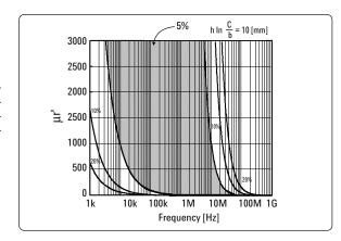
Figure 30. Permeability measurement accuracy (supplemental data)
