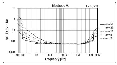
Figure 13. Loss tangent measurement accuracy (supplemental data)
