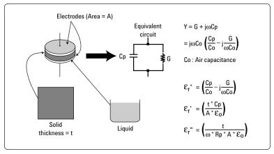
Figure 2. Parallel plate method
