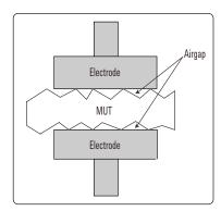
Figure 22. Rough-surfaced dielectric material
