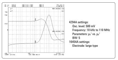
Figure 34. Low frequency response of MnZn ferrite core
