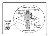
Figure 18. Structure of 16453A
