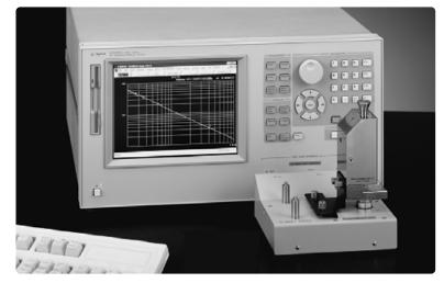
Applicable measurement instruments: E4991A (Option E4991A-002)\*
