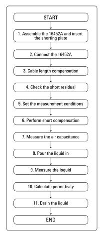
Figure 42. Measurement procedure flowchart for the 16452A  $\,$
