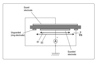
Figure 36. Surface resistivity
