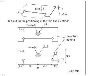
Figure 23. Fabricated thin film electrode's size
