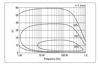
Figure 19. Permittivity measurement accuracy (supplemental data)
