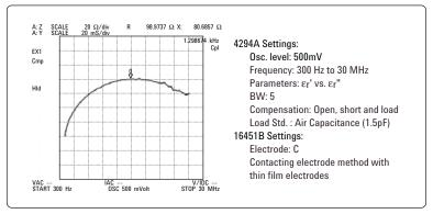
Figure 16. Cole-Cole plot of a ceramic material
