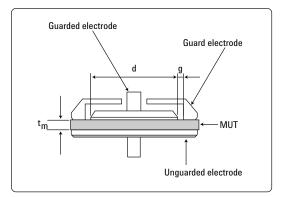
Figure 4. Contacting electrode method
