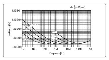
Figure 31. Loss tangent measurement accuracy (supplemental data)
