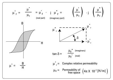
Figure 26. Definition of complex permeability (m\*)
