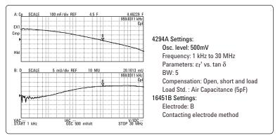
Figure 15. Frequency response of printed circuit board
