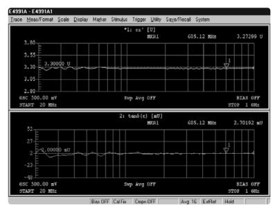
Figure 25. Frequency response of BT resin
