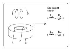
Figure 27. Method of measuring effective permeability
