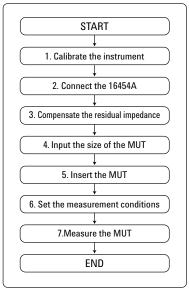
Figure 32. Measurement procedure flowchart for the 16454A
