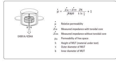
Figure 29. Structure of 16454A and measurement concept
