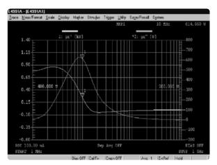
Figure 33. Frequency response of MnZn ferrite core
