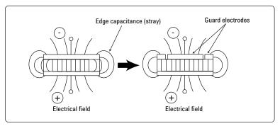
Figure 3. Effect of guard electrode
