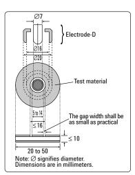
Figure 10. Electrode D dimensions
