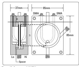
Figure 40. Structure of 16452A
