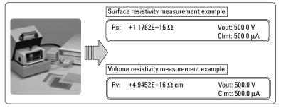
Figure 39. Surface and volume resistivity of polyimide
