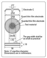
Figure 9. Electrode C dimensions
