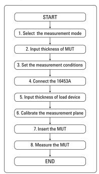
Figure 21. Measurement procedure flowchart for the 16453A
