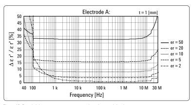
Figure 12. Permittivity measurement accuracy (supplemental data)
