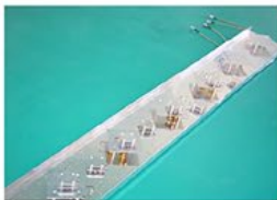
L-probe patch antenna 2G-3G base station
