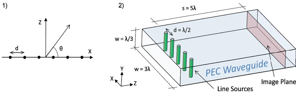
Figure 1. A diagram showing a generic antenna array (elements denoted by black dots).
