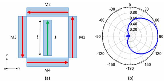
Fig. 1 An active Huygens surface (AHS) in free space. (a) A diagram showing metallic strips from which electric and magnetic dipoles are excited by driving currents through the green and red arrows, respectively. (b) The resultant antenna pattern when the electric and magnetic dipoles are excited with a ratio given in (1). Simulations are performed at a frequency of 3 GHz, with  $l = 5$  mm and  $S = 36$  mm<sup>2</sup>.
