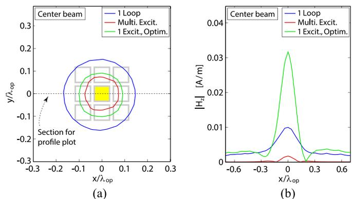
Fig. 2. Comparison of resulting beam for focusing obtained using single element excitation, multiple element excitation, and capacitor-optimized single element excitation. Panel (a) shows FWHM beamwidth contours of the beams, while panel (b) shows the profile of the magnetic field magnitude.
