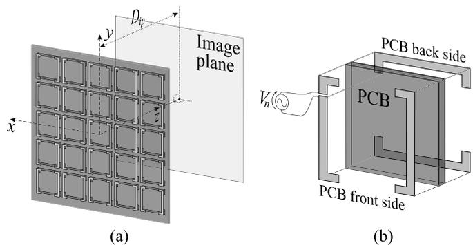
Fig. 1. Loop antenna array geometry. Panel (a) shows the entire array, and panel (b) shows the loop element structure.
