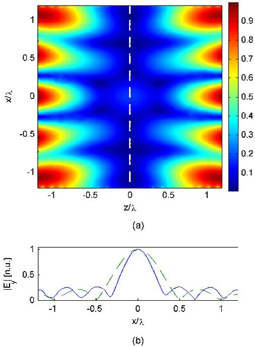
Fig. 4. Superscillation subwavelength focusing using Huygens metasurfaces. (a) A 2D plot of the electric field distribution within the cavity. Huygens metasurfaces are located across the four boundaries of the cavity; the fields are identically zero outside the cavity. The dashed line denotes the image plane  $z = 0$ . (b) The electric field profile along the image plane (blue, solid), the subwavelength focal width is 70% the width of the diffraction-limited curve (green, dashed).
