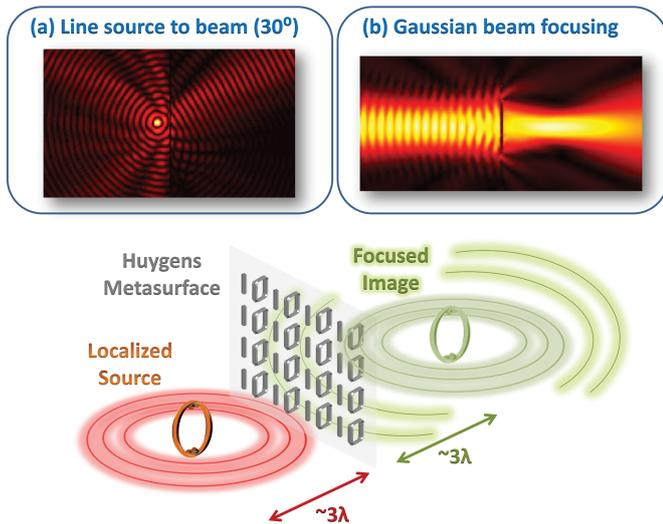
Fig. 3. Illustration of focusing using Huygens metasurface. Insets: HFSS simulated fields of passive HMS (a) converting electric line source fields into  $30^\circ$  directive beam [6]; (b) focusing a Gaussian beam [7].
