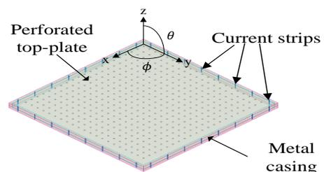
Fig. 1. The Huygens' box antenna with 32 active sources
