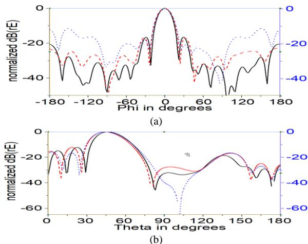
Fig. 3. Radiation Patterns: (a)  $\phi = 0^\circ$  plane (b)  $\theta = 45^\circ$  plane. Solid black line represents the patch array, red dashed line represents the Huygens' box antenna with 32 sources, blue dotted lines dashed line represents the Huygens' box antenna with 24 sources.
