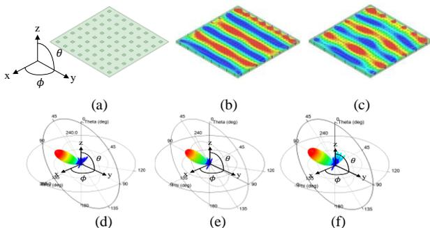
Fig. 2. (a)  $8 \times 8$  microstrip patch array (b-c) Huygens' Box Antenna with 32 sources and 24 sources respectively showing generated waves (d-f) radiation pattern of the microstrip patch array, Huygens' Box
