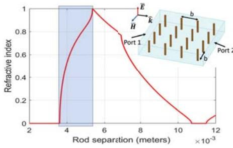
Fig. 1: Forming an effective artificial dielectric medium by arranging equispaced conductive rods. The plot relates  $n$  to spacing  $b$  at  $f = 28\text{GHz}$  and  $r = 0.25\text{mm}$ . The shaded portion has real  $n < 1$  at  $b < \lambda_0/2$ .  $\vec{E}$ ,  $\vec{H}$  and  $\hat{k}$  are the E-field, H-field and wave propagation direction respectively. The E-field is polarized along the direction of the rods.  $\epsilon_r$ ,  $\mu_r$  and  $n$  can be extracted using the S-parameters.
