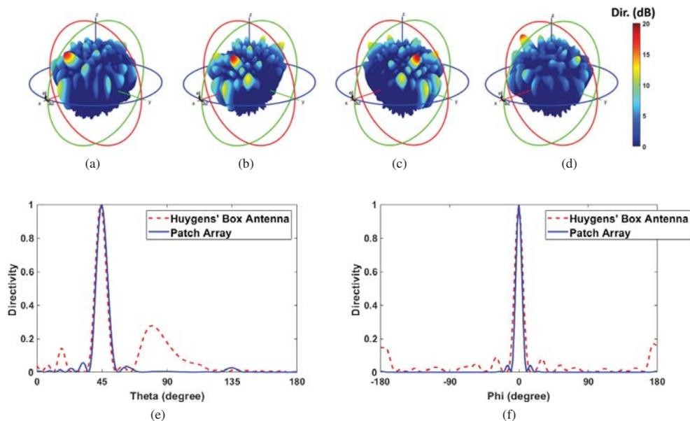
Fig. 3: Simulated radiation patterns. (a) - (d) shows radiated beams for elevation  $\theta = 45^\circ$  at  $\phi = 0^\circ$ ,  $\phi = 22.5^\circ$ ,  $\phi = 67.5^\circ$  and  $\phi = 275^\circ$  respectively. (e) 2D radiation patterns at  $\phi = 0^\circ$  plane (f) 2D radiation patterns at  $\theta = 45^\circ$  plane.
