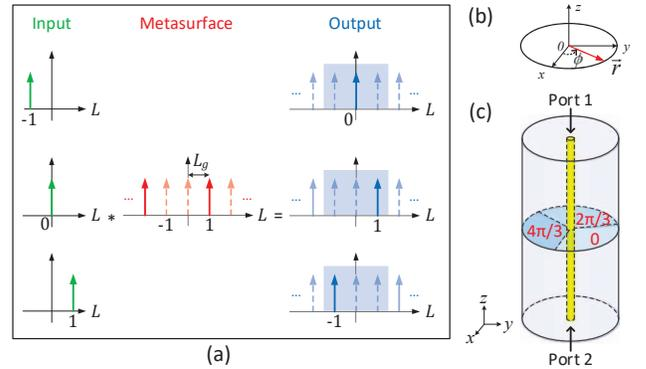
Fig. 3. (a) The  $L$ -space operation of a metasurface featuring the circulation of three modes with SAMs of  $-1$ ,  $0$ ,  $1$ . (b) SAM of an EM wave propagating along the  $+z$ -direction. (c) An ideal model designed to prove the concept of  $L$ -space mode circulation.
