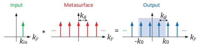
Fig. 1.  $k$ -space operation of a periodic metasurface that varies along  $y$ -direction. Arrows indicate the existence of diffraction modes.
