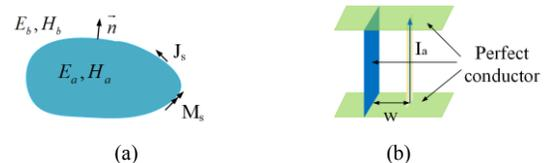
Fig. 1. (a) A diagram illustrating the equivalence principle. (b) A simple active Huygens' metasurface element with a perfect conductor.
