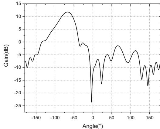
Fig. 8. The E-plane radiation pattern of the 2-D series-fed metasurface.
