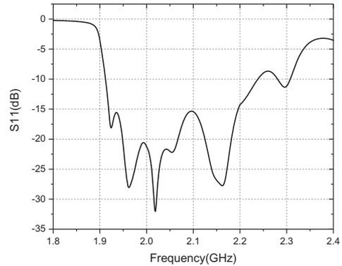
Fig. 5. The S parameter of the series-fed active metasurface.
