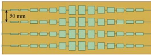
Fig. 7. The model of the 2-D series-fed metasurface.
