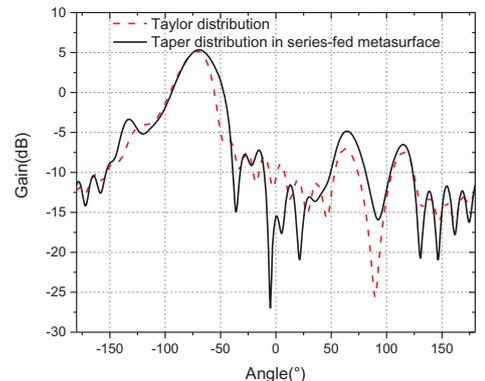
Fig. 6. The E-plane radiation pattern of the 1-D series-fed active metasurface and the radiation pattern of a corresponding antenna with the Taylor current distribution.
