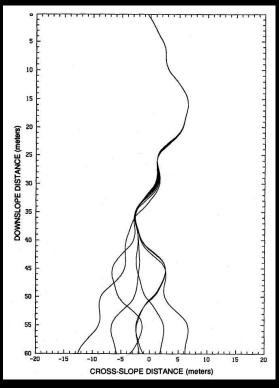
Diverging trajectories of 7 boards starting with same speed and spaced at 1mm intervals.
