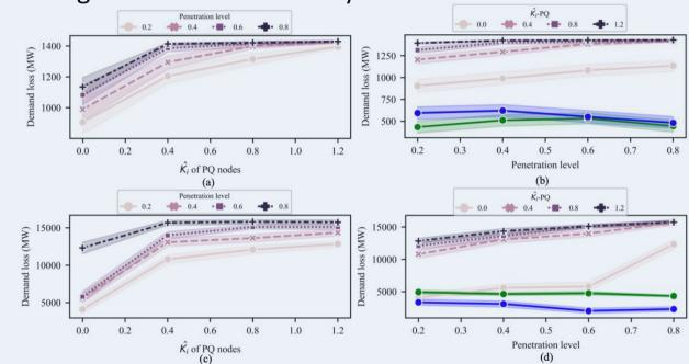
Influence of design parameter for droop controller and penetration level of frequency responsive inverter nodes on demand loss. Different percentages of PV buses are assigned as inverter nodes.
