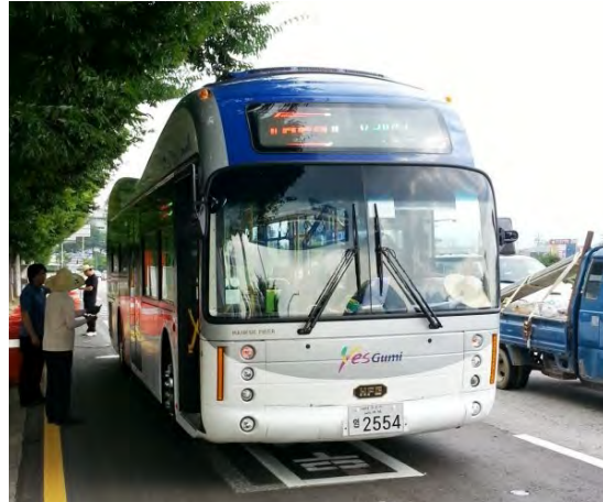
KAIST, Korea City of Gumi Air gap: 23 cm Power: 5x20 kW (2013)
