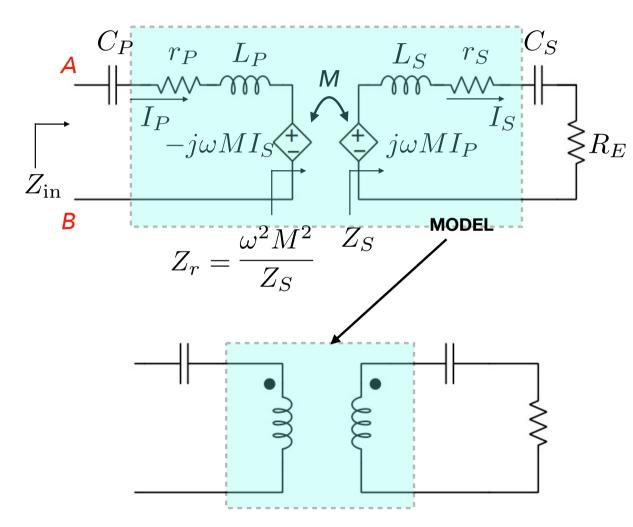
Secondary side efficiency  $\eta_S = \frac{R_E}{\Re[Z_S]} = \frac{R_E}{r_S + R_E}$ Primary side efficiency  $\eta_P = \frac{\Re[Z_r]}{\Re[Z_r] + r_P}$ Total efficiency  $\eta_T = \eta_P \eta_S$
