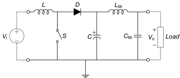
(b) Boost voltage converter with output filter
