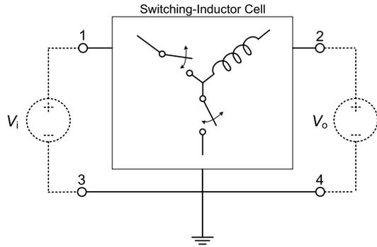
such that a closed-circuit continuous path will always exist for the flow of the inductor current. For this reason, this switching-inductor cell represents the minimum configurable switching-inductor structure possible. To qualify for a lossless conversion process, the switching-inductor cell must be implemented with an input voltage source together with an output voltage sink (see Fig. 1.2), which forms the basis for a voltage-to-voltage converter.
