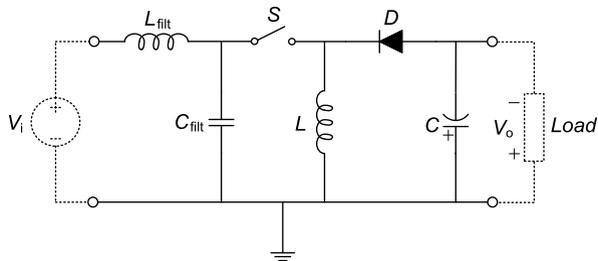
(c) Buck-boost voltage converter with input filter
