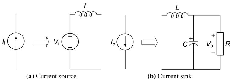
Fig. 1.12 (a) Current source replaced by an equivalent of voltage source and series inductor and (b) current sink replaced by a resistor–capacitor sink and series inductor
