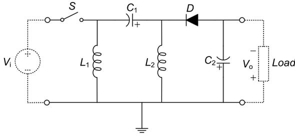
**Fig. 1.16** The “missing” fourth-order converter
