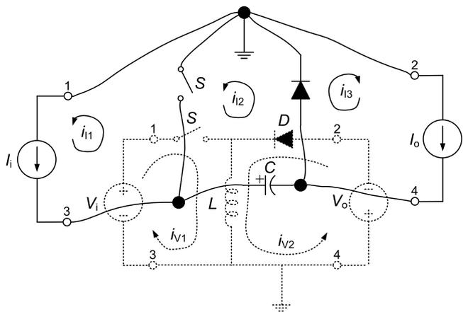
Fig. 1.11 Dual transformation of a buck–boost converter
