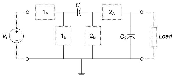
Fig. 1.14 Generic fourth-order converter with two-inductor–two-switch cutset
