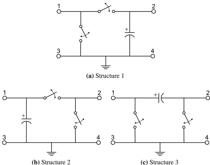
Fig. 1.7 The three possible configurations of the switching-capacitor cell
