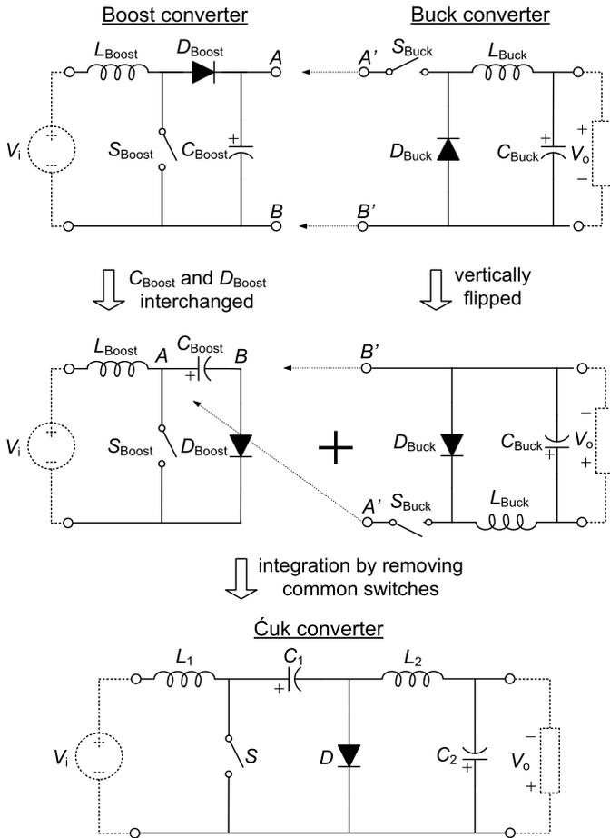
**Fig. 1.19** Ćuk converter derived from the cascade of a boost and a buck converter
