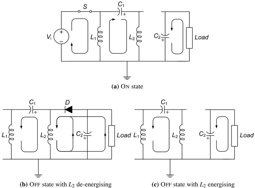
**Fig. 1.17** The three possible operating states of the “missing” fourth-order converter
