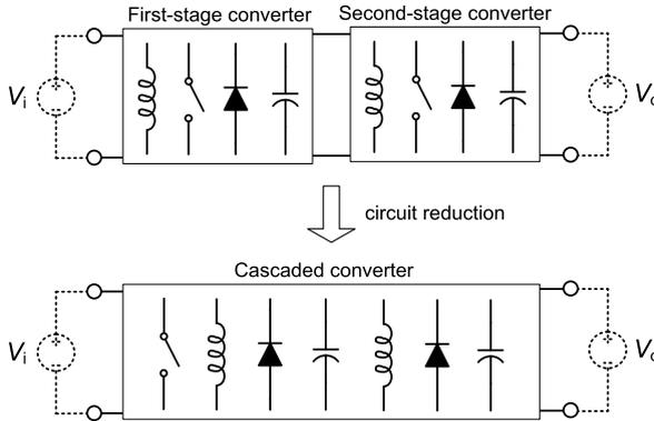
**Fig. 1.18** Fourth-order voltage converter derived from the cascade of two second-order voltage converters
