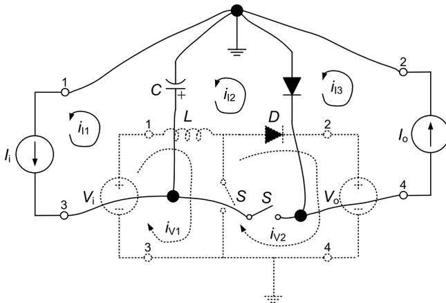
Fig. 1.10 Dual transformation of a boost converter
