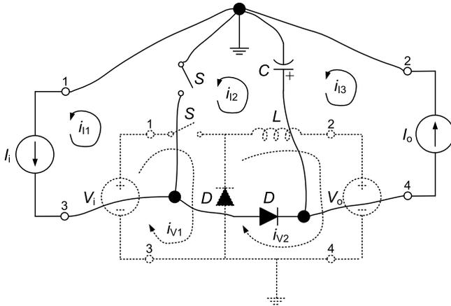
Fig. 1.9 Dual transformation of a buck converter
