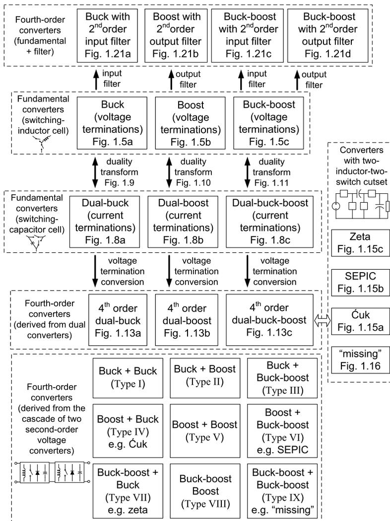
Fig. 1.1 Overview of the relationships of converter topologies
