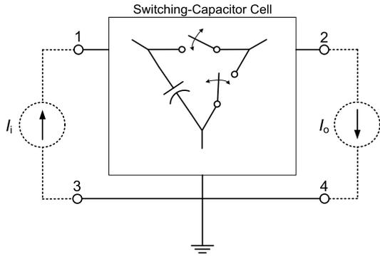
synchronised to operate complementarily to ensure that there is no circumstance that the capacitor has a direct short circuit. This gives the minimum configurable switching-capacitor structure. For lossless energy transfer, the switching-capacitor cell must be implemented with an input current source and an output current sink. This forms the basis for the current-to-current converters.
