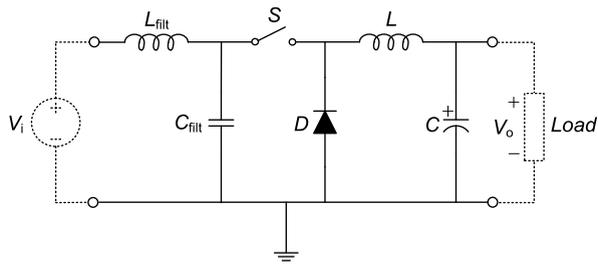
(a) Buck voltage converter with input filter
