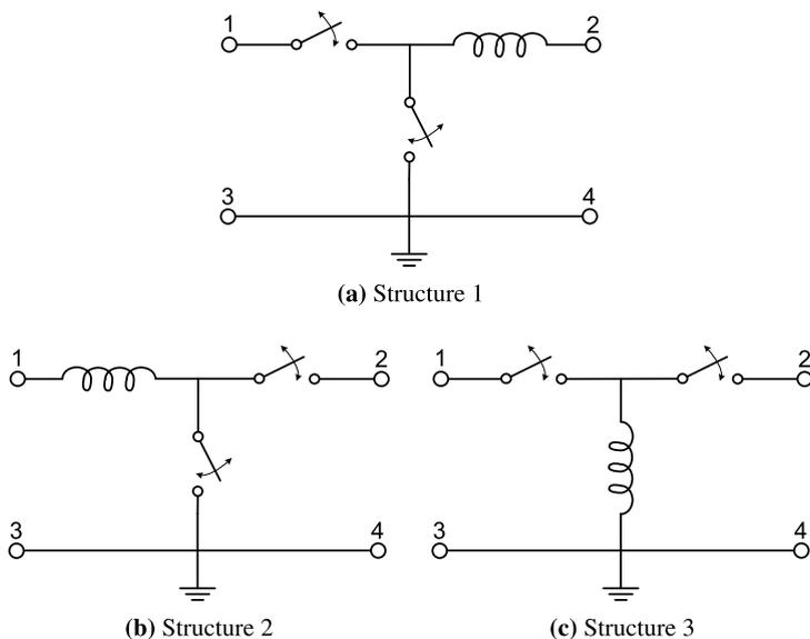
**Fig. 1.3** The three possible configurations of the switching-inductor cell
