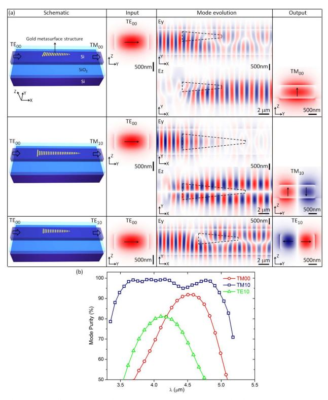
Fig. 4 Mid-infrared waveguide mode converters and polarization rotator based on plasmonic gradient metasurfaces. (a) Simulated device performance. The first column shows device schematics. The gradient metasurface structures consist of gold phased array antennas
