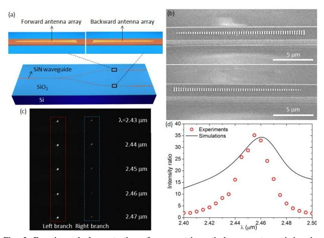
Fig. 3 Experimental demonstration of asymmetric optical power transmission in waveguides patterned with gradient metasurface structures. (a) Schematic of fabricated devices consisting of a Y-branch waveguide and two gradient metasurface structures patterned
