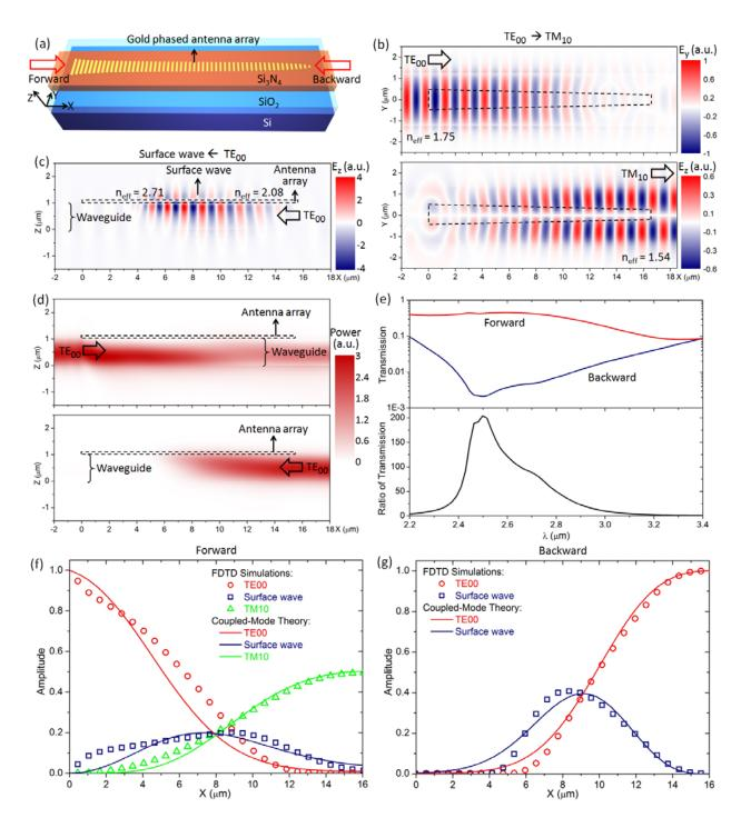
Fig. 2 Asymmetric optical power transmission in waveguides patterned with gradient metasurface structures. (a) Schematic of a device working around  $\lambda = 2.5 \mu m$ . The  $Si_3N_4$  waveguide is 2.5  $\mu m$  in width and 1.0  $\mu m$  in thickness. The center-to-center distance between adjacent antennas is 300 nm. The length of the antenna array is 16.5  $\mu m$ . The detailed design parameters are provided in Supplementary Section V. (b)-(c) Full-wave simulations showing
