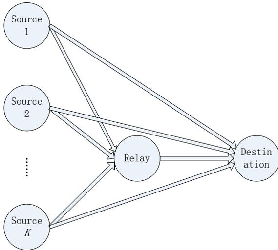
Fig. 1. The multiple-access relay channel with  $K$  users
