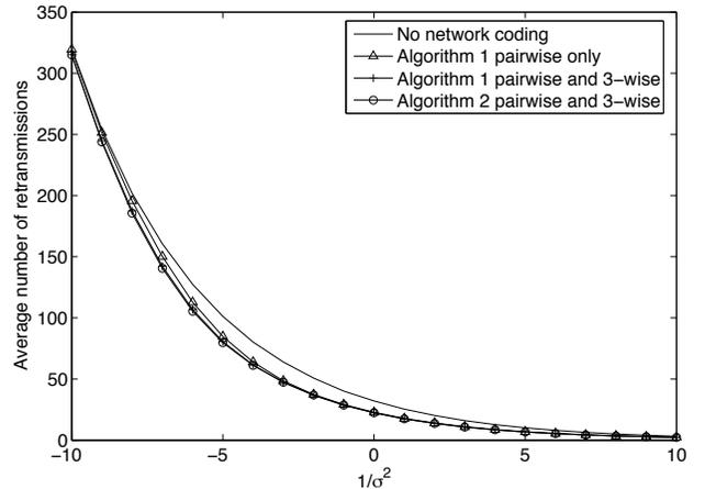
Fig. 4. Relay-to-destination channel is block Rayleigh faded, and the distance from relay to destination is the same as source to destination,  $\Gamma_{th}=3\text{dB}$ , 32 users
