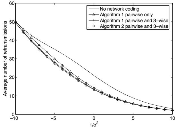
Fig. 3. Relay-to-destination channel is block Rayleigh faded, and relay is at the middle of the users and the destination,  $\Gamma_{th}=3\text{dB}$ , 32 users
