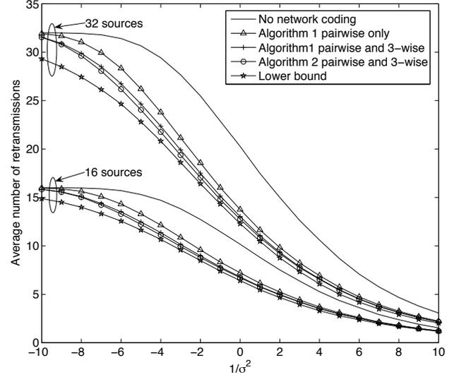
Fig. 2. Ideal relay-to-destination channel,  $\Gamma_{th}=3\text{dB}$ , 16 and 32 sources
