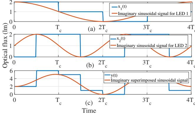
Fig. 2: The codewords and their corresponding imaginary analog sinusoidal signals at (a) LED 1 (b) LED 2 (c) receiver.
