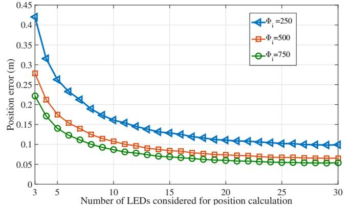
Fig. 8: Position error versus the number of LEDs considered for position calculation, in the space dimensions and LEDs configuration in Setup 2 shown in Fig. 3(b).
