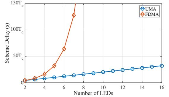
Fig. 4: The scheme delays of UMA and FDMA vs the number of LEDs.
