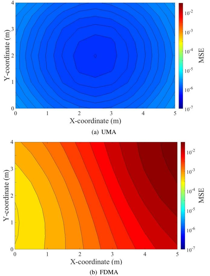
Fig. 6: MSEs of UMA and FDMA vs receiver position in Setup 1.
