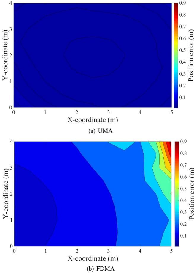
Fig. 7: Position errors of UMA and FDMA vs receiver position in Setup 1.
