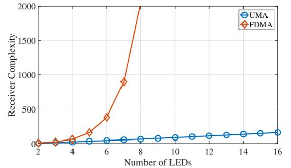
Fig. 5: The receiver complexity of UMA and FDMA vs the number of LEDs.
