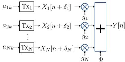
Fig. 1. Transmitters want to broadcast different messages. They are suffering from random delays due to the different activation time. The superposition of ambient light and the transmitted signals is received by the receiver.
