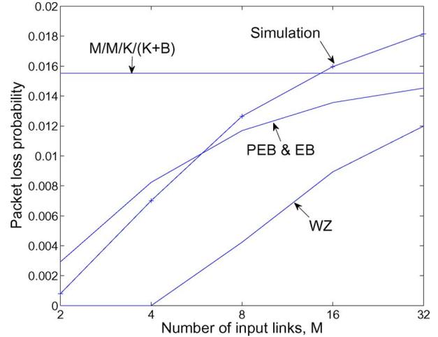
Fig. 7. Packet loss probability versus number of input ports, for  $K = 1$  output ports,  $B = 3$  packet buffer, and load  $A = 0.4$ .
