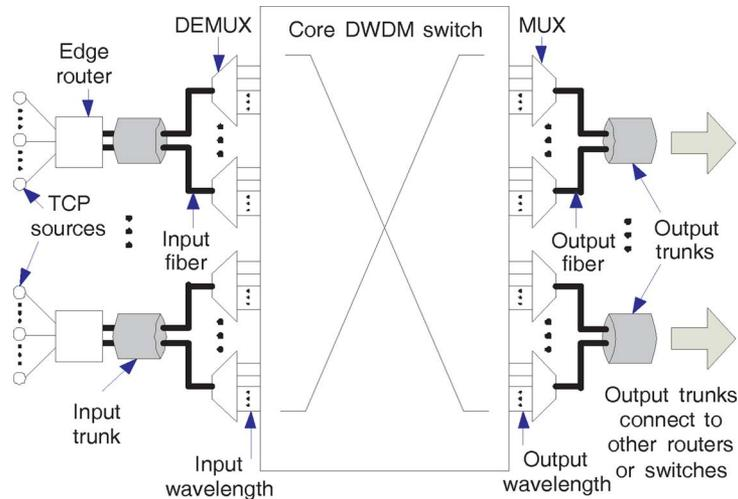
Fig. 1. Network topology of an optical network with a bottleneck symmetric switch.
