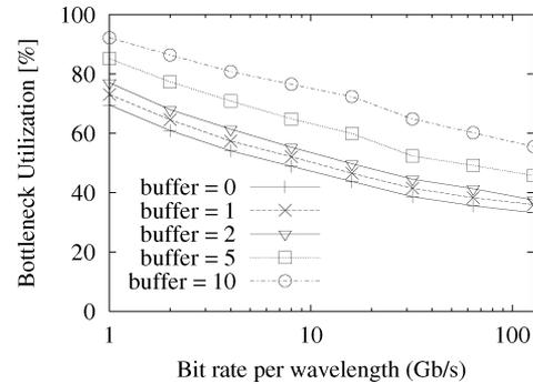
Fig. 11. Percentage bottleneck utilization as a function of link bit rate (80 input ports, 20 output ports and 20,000 TCP flows).
