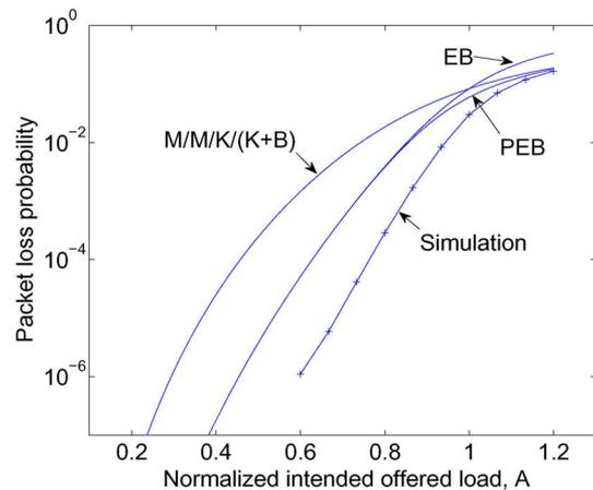
(b)  $M = 2$  input ports,  $K = 1$  output ports,  $B = 10$  packet buffer
