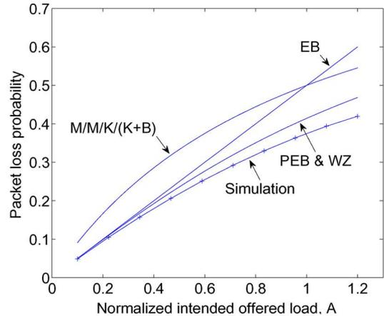
(a)  $M = 2$  input ports,  $K = 1$  output ports,  $B = 0$  packet buffer
