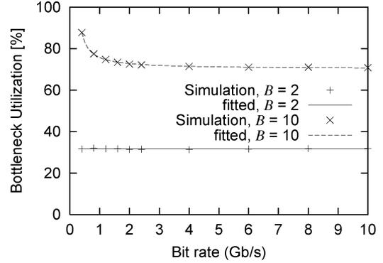
Fig. 3. Curve fitting of bottleneck utilization,  $B = 2$  and 10 [packets].
