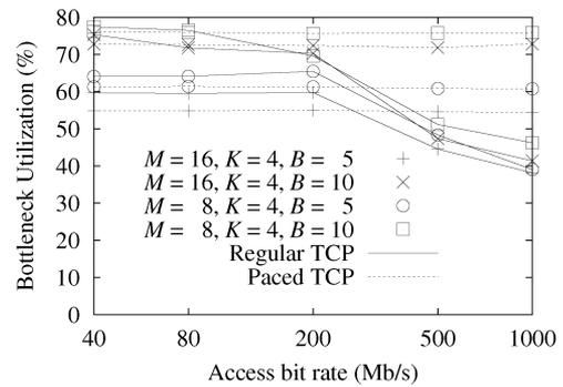
Fig. 12. Effect of access bit rate on bottleneck utilization of regular versus paced TCP over a 1 Gbit/s bottleneck.
