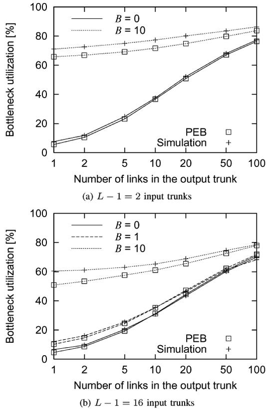
Fig. 9. Bottleneck utilization versus number of links per trunk ( $K$ ).
