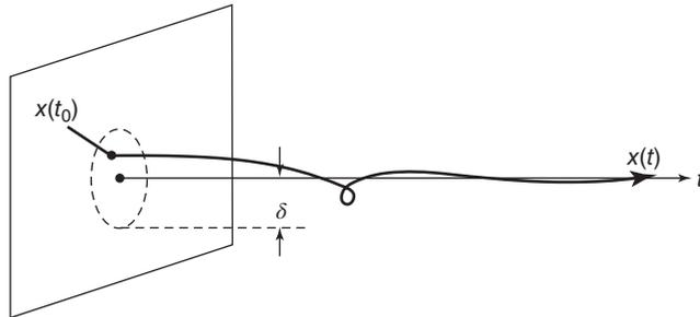
**Figure 5** Geometric meaning of the asymptotic stability.
