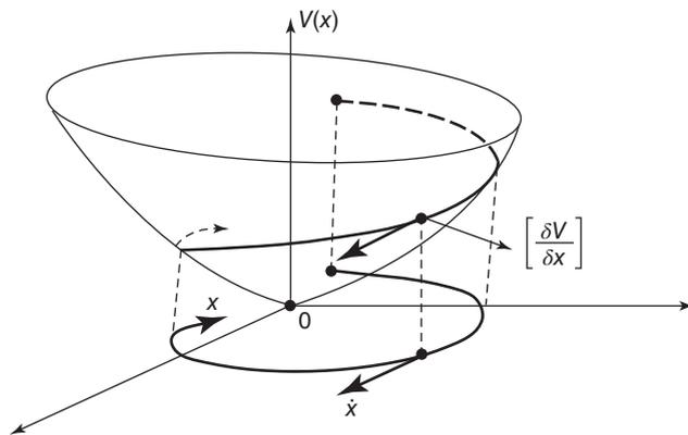
**Figure 9** Geometric meaning of the Lyapunov function.
