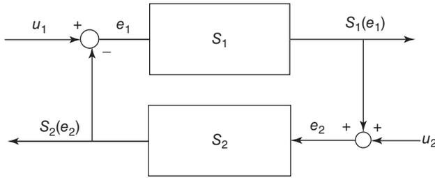
**Figure 3** A typical closed-loop control systems.
