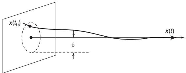
**Figure 6** Geometric meaning of the exponential stability.
