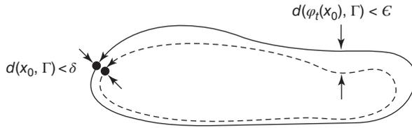
Figure 7 Geometric meaning of the orbital stability.
