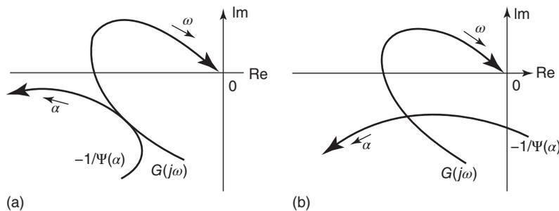
**Figure 16** Graphical describing function analysis.
