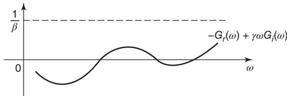
Figure 14 Geometric meaning of the Popov criterion.
