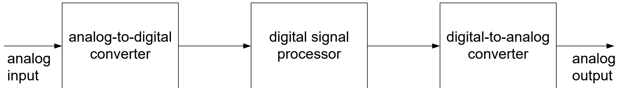
Fig.1.12: Digital processing of analog signal
