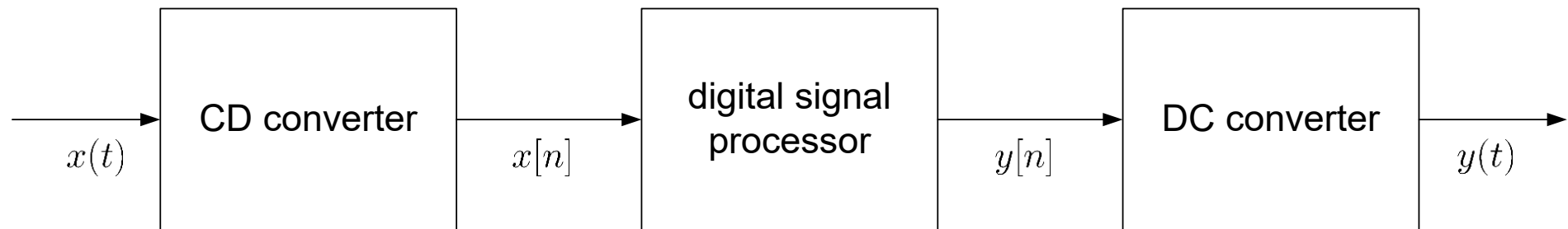
Fig.4.8: Ideal digital processing of analog signal
