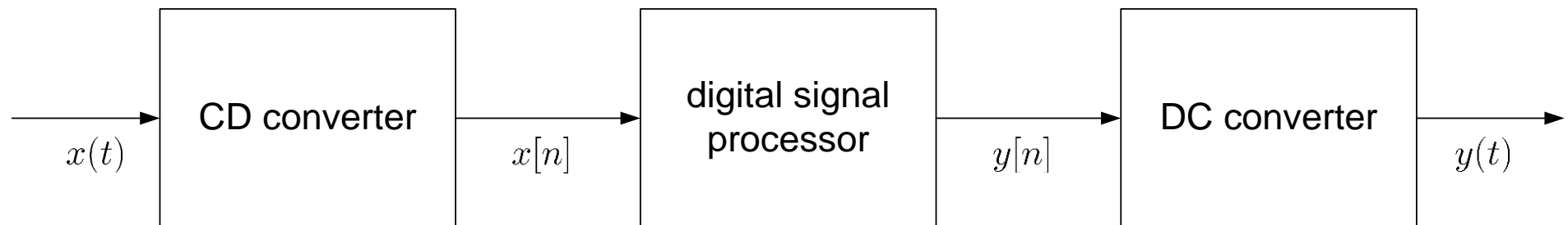
Fig.4.8: Ideal digital processing of analog signal
