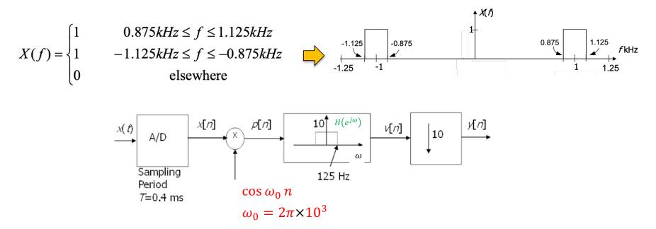
•  $H(e^{j\omega})$  is an ideal lowpass filter (gain=10) with cut-off frequency  $f_c = 125$  Hz. Sketch, one above another,  $|X(e^{j\omega})|$ ,  $|P(e^{j\omega})|$ ,  $|V(e^{j\omega})|$ ,  $|Y(e^{j\omega})|$  against  $\omega$ .
