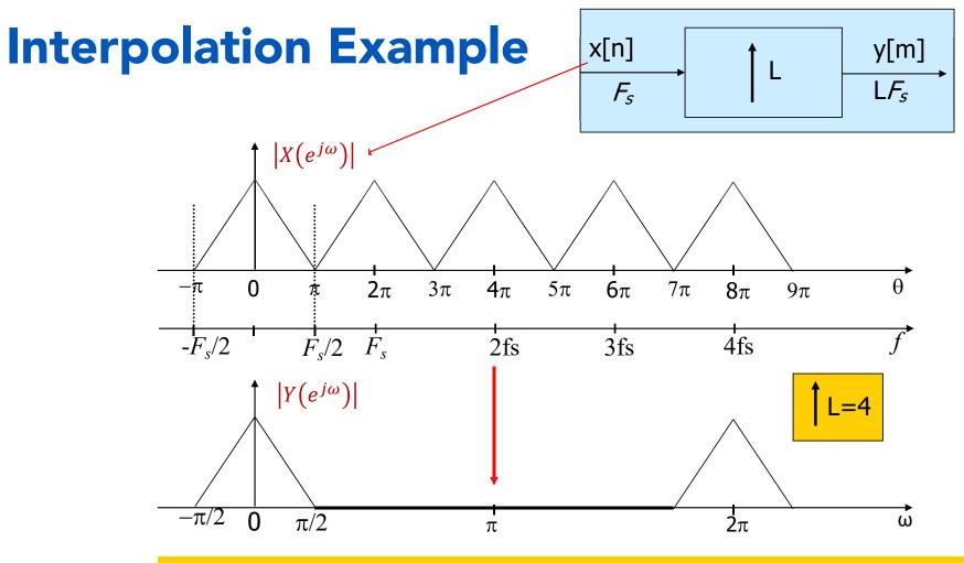
Sampling frequency of  $y[m] = 4F_s$ ; Signals must be band limited to  $2F_s$
