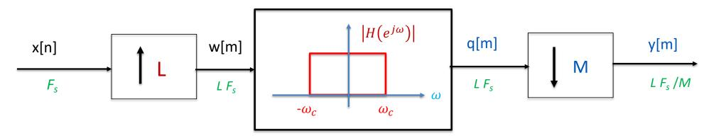
• The two Digital Lowpass Filters,  $H_1(e^{j\omega})$  and  $H_2(e^{j\omega})$  can be combined into a single lowpass filter  $H(e^{j\omega})$  with cut-off frequency  $\omega_c$ :
