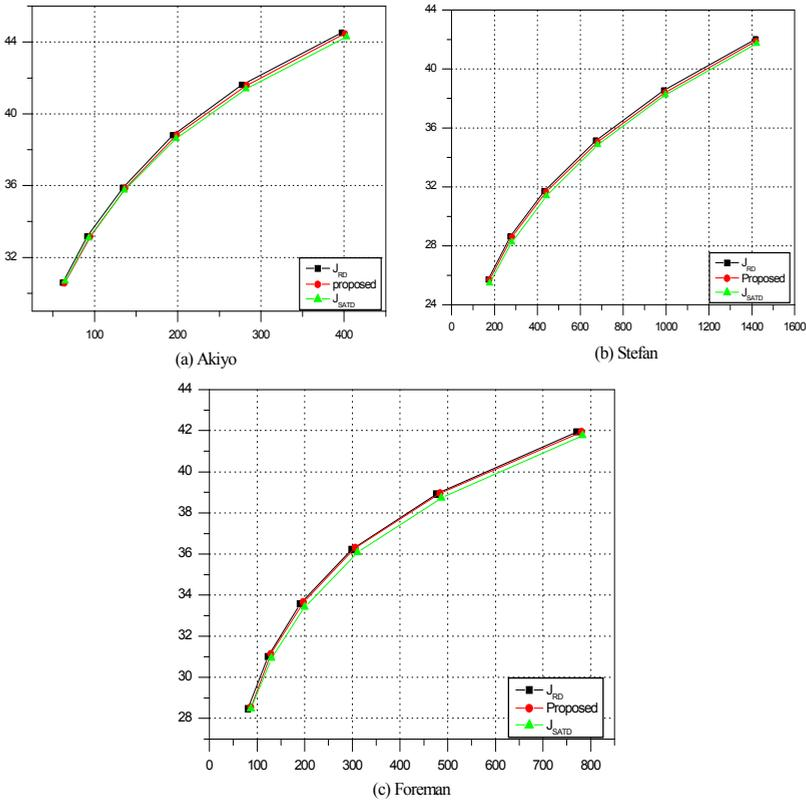
Fig. 15. RD performance with CABAC entropy coding method
