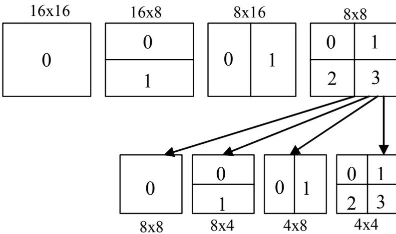
Fig. 2. Variable block sizes of macroblock of INTER mode
