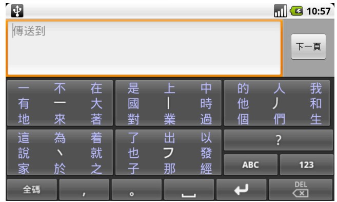
Fig. 5: The proposed dynamic keypad with eight most likely characters displaying around the stroke keys.
