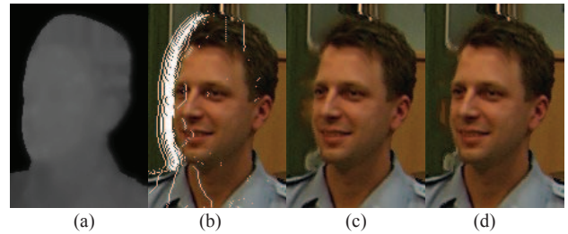
Fig. 5: Synthesized view using adaptive filter in depth map preprocessing: (a) Preprocessed Depth map by adaptive filter, (b) Warpped Image, and (c) Synthesized Image using Inpainting hole filling, (d) Synthesized Image using multidirectional extrapolation.
