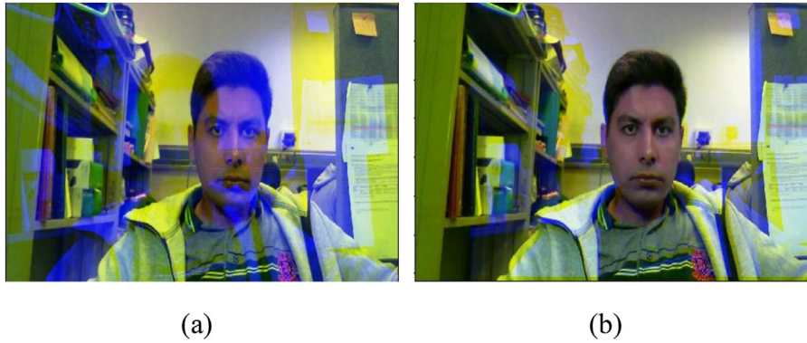
Fig. 3. Result of single point matching. (a) Image before alignment: The blue channel of the left camera image is visible. (b) The image after alignment using single point matching.
