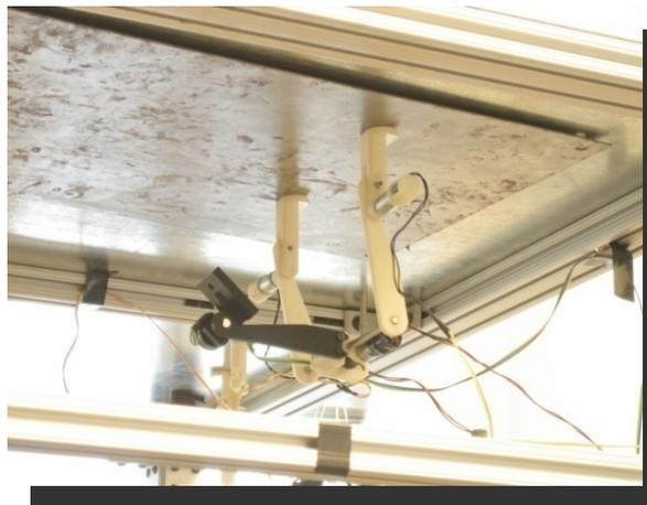
Pendulum robot swings over aircraft and tracks the surface profile for inspection
