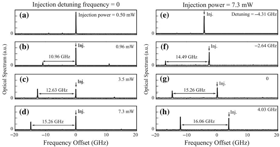
**Fig. 2** Optical spectrum of the slave laser subjected to optical injection. The frequency axes are offset to the free-running frequency of the slave laser. **(a–d)** Injection power varies while the detuning is kept at zero. **(e–h)** Injection detuning varies while the injection power is kept constant at 7.3 mW. The arrows indicate the injected optical frequency component
