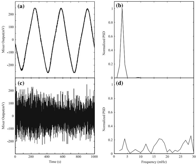
**Fig. 5** Mixer output for  $f_{\text{RF}} = 17$  GHz. The target moves away from the detector at  $26 \mu\text{m/s}$ . The Doppler shift frequency is 3 mHz: **(a)** Doppler measurement with locked period-one state, **(b)** the corresponding normalized power spectrum (PSD), **(c)** Doppler measurement with unlocked period-one state, and **(d)** the corresponding normalized PSD
