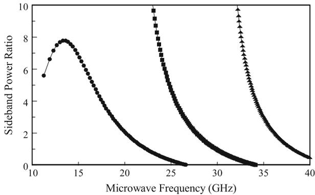
**Fig. 3** Optical power ratio of the generated sideband to the carrier. The injection strength is varied to tune the microwave frequency while the injection detuning is kept at 10 GHz (●), 20 GHz (■), and 30 GHz (▲), respectively
