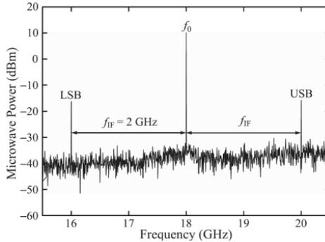
**Figure 4.** Power spectrum of the slave laser under P1 oscillation at  $f_0 = 18$  GHz and current modulation at  $f_{IF} = 2$  GHz. The input current modulation power is  $P_{IF} = -4$  dBm. Frequency up-conversion from  $f_{IF}$  to  $f_0 \pm f_{IF}$  is observed.
