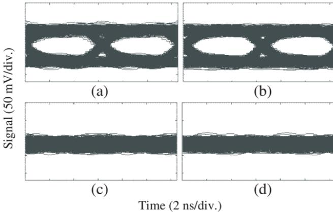
**Figure 7.** Eye diagrams of the data recovered at (a) 16-GHz LSB with optical injection. (b) 20-GHz USB with optical injection. (c) 16-GHz LSB without optical injection. (d) 20-GHz USB without optical injection.
