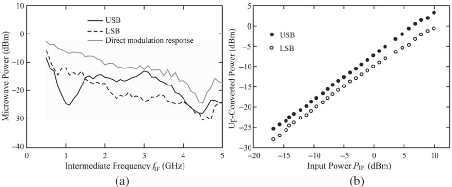
**Figure 5.** (a) Up-conversion power from the photonic microwave mixing of  $f_{IF}$  and  $f_0 = 18$  GHz. The solid and dashed dark curves correspond to the USB and the LSB, respectively. For comparison, the gray curve is the direct modulation response of the slave laser. Modulation power is kept at  $P_{IF} = -4$  dBm. (b) The USB and LSB power versus  $P_{IF}$  at  $f_{IF} = 2$  GHz.
