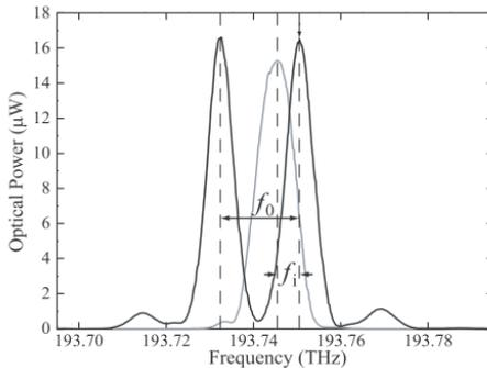
**Figure 2.** Optical spectrum of the emission from the slave laser under no current modulation. The gray curve is obtained without optical injection. The black curve is obtained with optical injection of  $f_i = 5$  GHz and  $P_i = 5.25$  mW. The slave laser exhibits P1 oscillation of  $f_0 = 18$  GHz. (Resolution bandwidth = 7.5 GHz).
