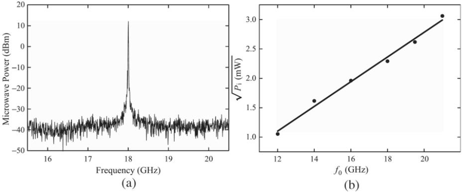
**Figure 3.** (a) Power spectrum of the slave laser under P1 oscillation at  $f_0 = 18$  GHz. No current modulation is applied. (b) Tunability of  $f_0$  by varying  $P_1$  under constant  $f_i = 5$  GHz.
