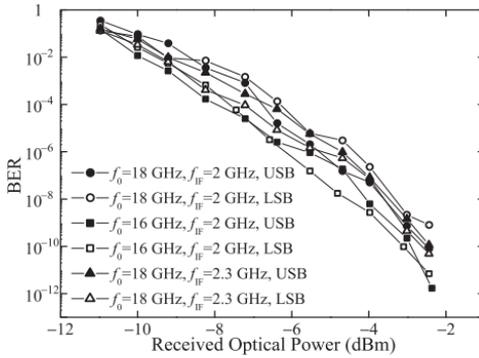
**Figure 8.** BER of the system under different P1 oscillation frequencies  $f_0$  and intermediate frequencies  $f_{IF}$ . Data rate = 155 Mbps.
