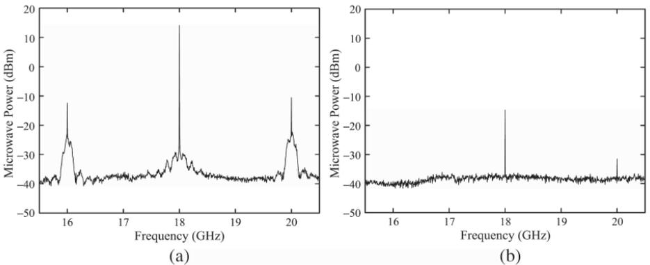
**Figure 6.** Power spectrum of the slave laser under current modulation at  $f_0 = 18$  GHz and  $f_{IF} = 2$  GHz. The modulation at  $f_{IF}$  carries BPSK data at 155 Mbps. (a) Up-converted signal when optical injection is applied. (b) Up-converted signal when optical injection is removed.
