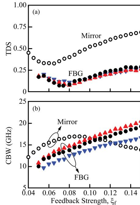
Fig. 7. Numerical results of (a) TDS and (b) effective bandwidth for the chaotic signals as functions of the feedback strength  $\xi_f$ . FBGs of bandwidths  $f_{BW} = 13$  GHz, 28 GHz, and 40 GHz are considered in closed down-triangles, closed circles, and closed up-triangles, respectively. For comparison, the open circles are obtained when the FBG is replaced by a mirror.
