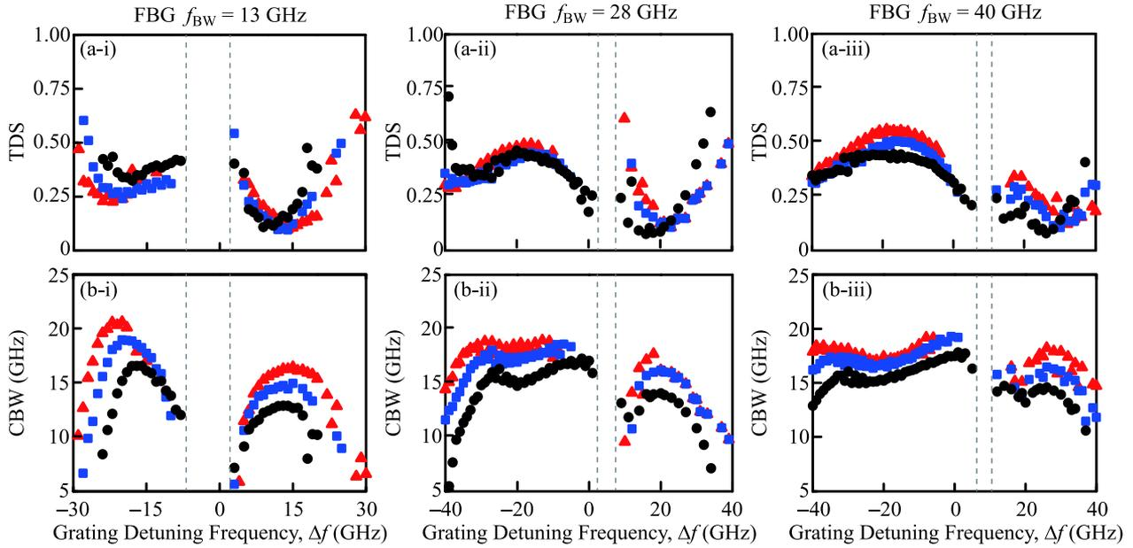
Fig. 6. Numerical results of (a) TDS and (b) effective bandwidth for the chaotic signals as functions of the FBG detuning frequency  $\Delta f$ . The feedback strength is fixed at  $\xi_f = 0.078$  (circles), 0.10 (squares), and 0.12 (triangles), respectively. The FBG bandwidth  $f_{BW} =$  (i) 13 GHz, (ii) 28 GHz, and (iii) 40 GHz, respectively.
