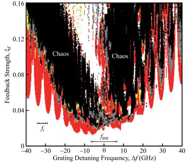
Fig. 3. Mapping of the output intensity dynamics in the parameter space of feedback strength  $\xi_f$  and grating detuning frequency  $\Delta f$ . The laser output intensity is stable (white), period-one oscillatory (red), quasi-periodic pulsating (gray), period-doubled oscillatory (yellow), and chaotic (black) in the different colored regions. The length of the FBG corresponds to  $f_l = 5$  GHz. The bandwidth of the FBG is  $f_{BW} = 13$  GHz.
