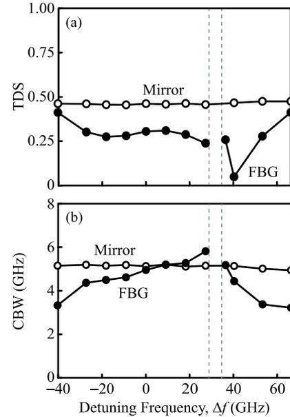
Fig. 9. Experimental results in closed symbols for (a) TDS and (b) effective bandwidth for the chaotic signals as functions of the FBG detuning frequency  $\Delta f$ , as varied by adjusting the free-running laser frequency. The FBG has a bandwidth of  $f_{BW} = 56$  GHz. For comparison, the open symbols are obtained when the FBG is replaced by a mirror. The feedback strength is fixed at  $\xi_f = 0.06$ .
