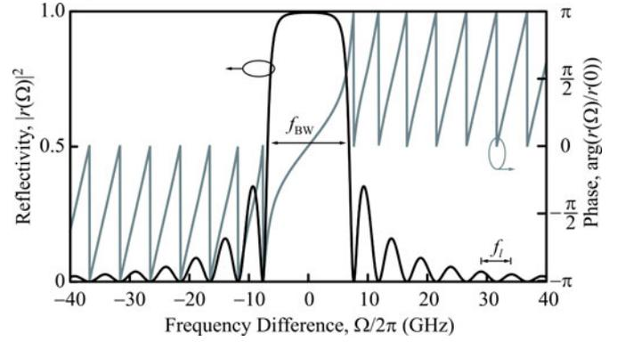
Fig. 2. FBG reflectivity spectrum  $|r(\Omega)|^2$  (black) and phase spectrum  $\arg(r(\Omega)/r(0))$  (gray). The frequency axis is centered at the Bragg frequency. The grating has a length of  $l = 20$  mm for  $f_l = 5$  GHz. Its FWHM bandwidth is  $f_{BW} = 13$  GHz.
