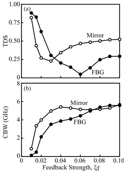
Fig. 10. Experimental results in closed symbols of (a) TDS and (b) effective bandwidth for the chaotic signals as functions of the feedback strength  $\xi_f$ . The FBG bandwidth is  $f_{\text{BW}} = 56$  GHz. For comparison, the open symbols are obtained when the FBG is replaced by a mirror.
