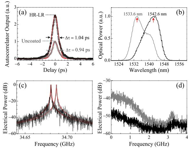
Fig. 2. (a) Autocorrelation pulse trace, (b) optical spectrum, (c) power spectrum at the mode-locking repetition frequency, and (d) power spectrum at the baseband. The power spectra are normalized to their respective peaks at the repetition frequency. Gray, original uncoated laser. Black, HR–LR-coated laser.
