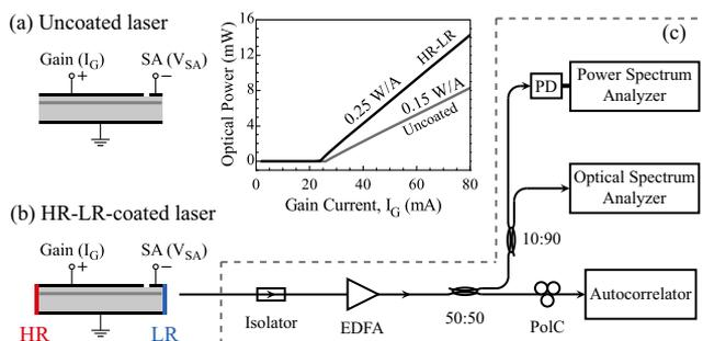
Fig. 1. (a) Original uncoated laser. (b) HR-LR-coated laser for ACPML. (c) Setup for mode-locked pulses characterization. PolC, polarization controller; PD, photodetector. Inset: Average optical output power versus gain section current for the uncoated laser (gray) and HR-LR-coated laser (black) when the SA is unbiased.
