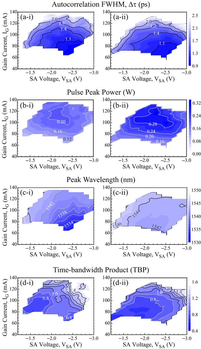
Fig. 3. (a) Autocorrelation FWHM  $\Delta\tau$ , (b) estimated peak power, (c) emission peak wavelength, and (d) TBP for the original uncoated laser (left column) and the HR-LR-coated laser (right column). Only mode-locked regions with amplitude noise below 0 dB and  $\Delta\tau < 2.5$  ps are shown.
