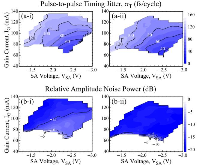
Fig. 4. (a) Pulse-to-pulse timing jitter  $\sigma_T$  and (b) relative amplitude noise power for the original uncoated laser (left column) and the HR-LR-coated laser (right column). Only mode-locked regions with amplitude noise below 0 dB and  $\Delta\tau < 2.5$  ps are shown.
