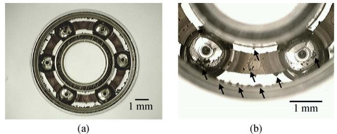
Fig. 8. (a) Failed bearing. (b) Close up of (a). Arrows indicate tiny metal particles detached from bearing surfaces.
