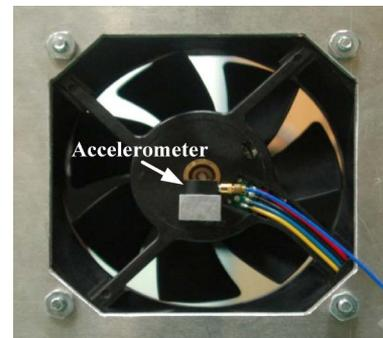
Fig. 6. Fan and accelerometer.
