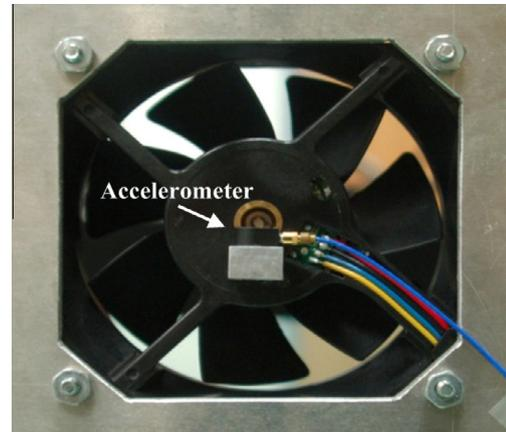
Fig. 3. Cooling fan and accelerometer (Jin et al., 2012; Miao, Azarian, et al., 2011).
